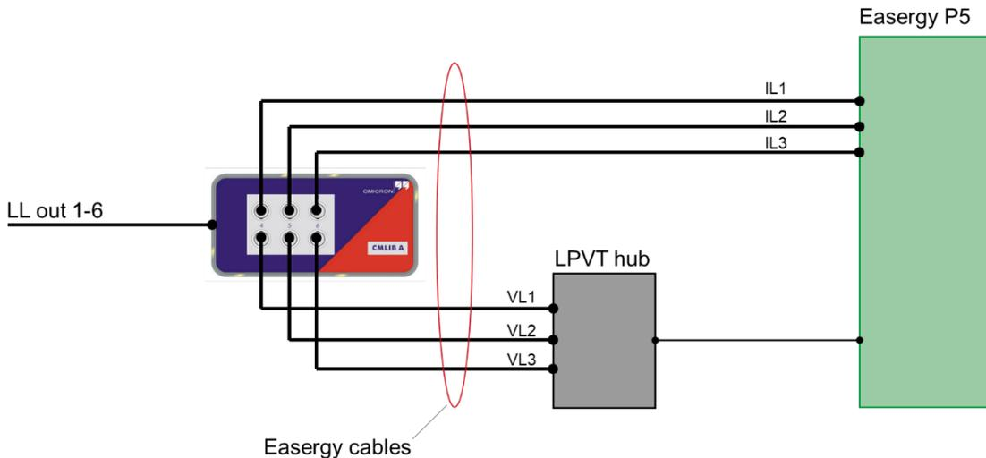
Figure 8: Test setup with CMLIB A and Easergy cables
