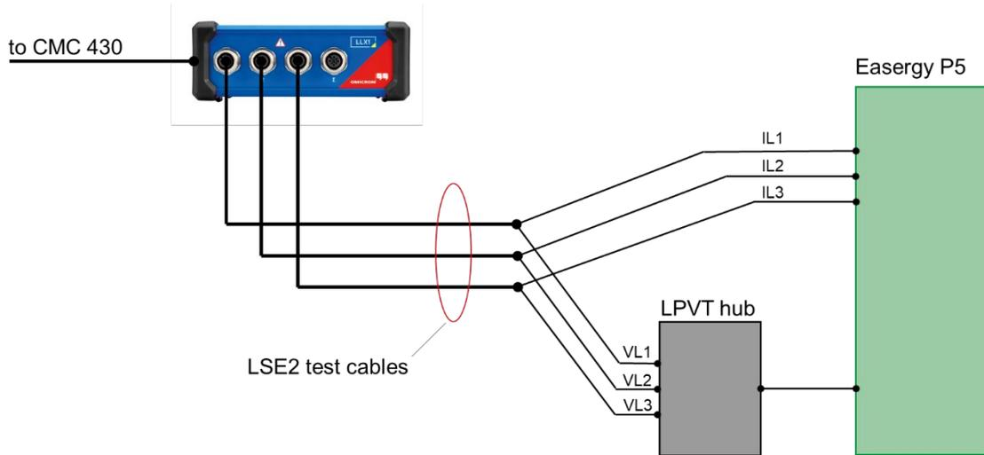
Figure 11: Test setup with LLX1 and LSE2 test cables
