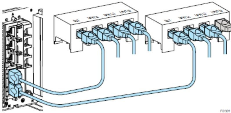
Figure 3: LPVT hub connector connected to Easergy P5 protection relay
