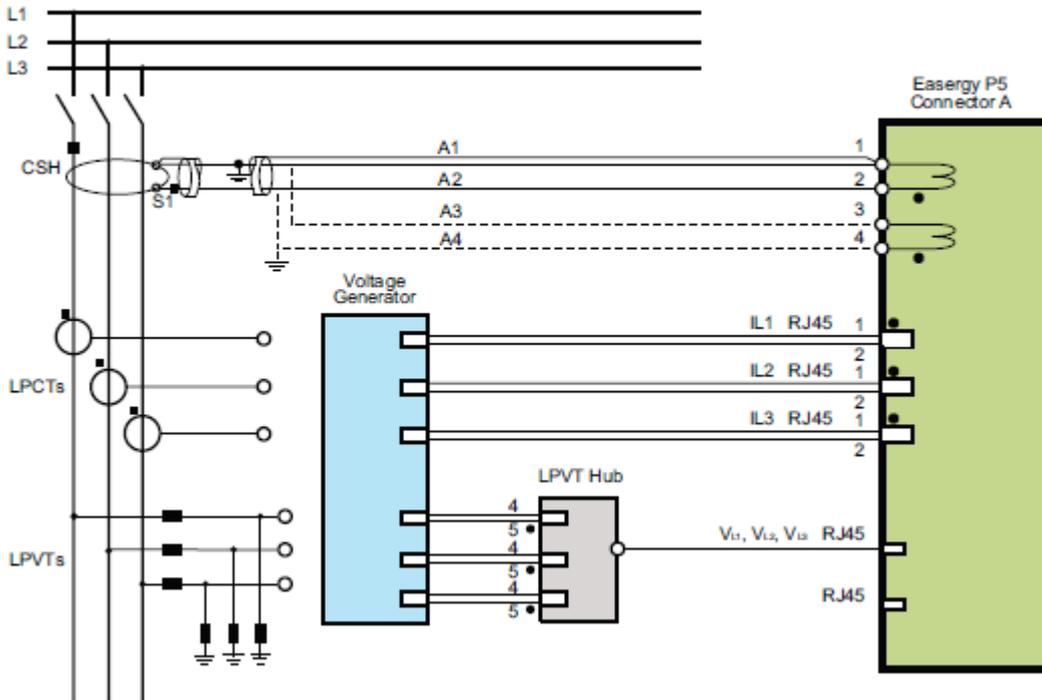
Figure 7: Connection diagram for testing from Easergy P5 User Manual
