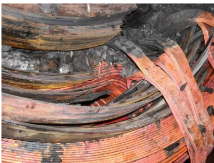
Figure 9 - Observed Winding Movement LV Winding Phase B
