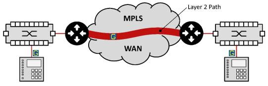
Figure 2: GOOSE communication between substations via a layer 2 path
