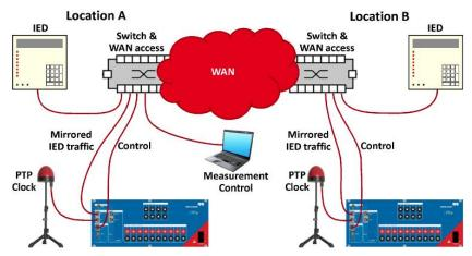
Figure 4: Propagation time measurement over a WAN
