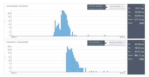
Figure 6: One-way propagation delays between Texas and Austria
