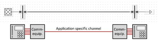
Figure 1: Conventional communication aided line protection scheme
