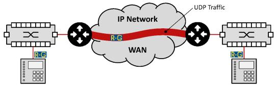
Figure 3: Routable GOOSE communication between substations via an IP route
