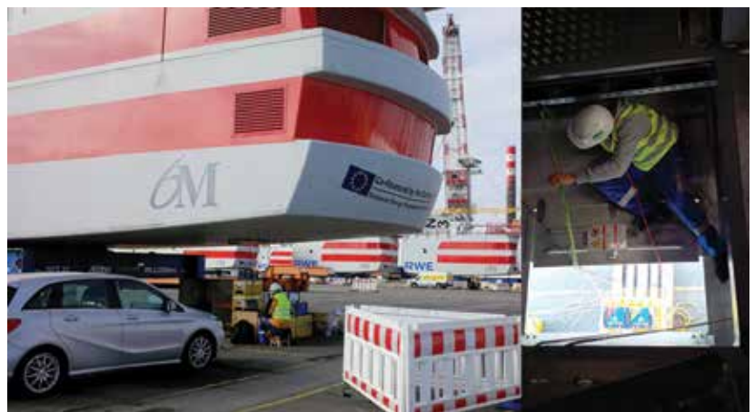
Figure 9: On-Site PD Measurements during Induced Testing of an Installed Transformer
