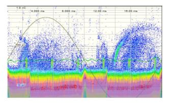
Figure 11 PRPD of cable, recorded using a monitoring system.
