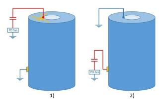
**Figure 9** 1) Connection of the coupling capacitor at the top of the winding, surface discharges 2) Coupling capacitor and ground swapped, free of PD.
