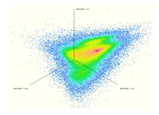
Figure 5 3CFRD of a transformer with multiple PD sources
