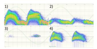
**Figure 6** 1) Complete PRPD, 2) Background noise, 3) Corona discharge, 4) Advanced surface discharge, after separation using 3CFRD.
