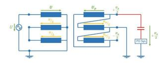
**Figure 4** Test setup of a single-phase induced voltage test for a Dyn transformer.
