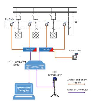
FIGURE 4 TEST SETUP FOR A SYSTEM-BASED BUSBAR PROTECTION TEST
