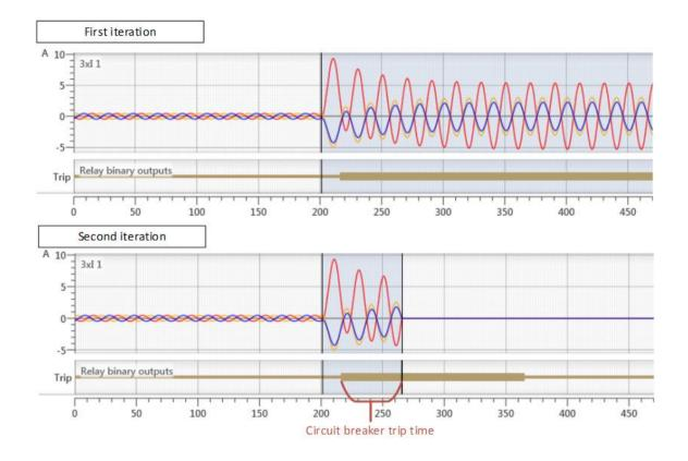
FIGURE 5: EXEMPLARY ITERATIVE CLOSED-LOOP SEQUENCE
