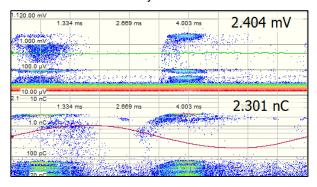
Figure 16: Simultaneously measured PD pattern of the UHF system (top) and conventional PD detector at the bushing tap (bottom)
