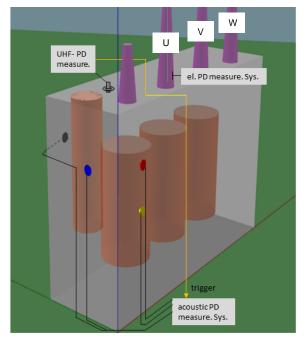
Figure 18: Test setup (UHF, el. and acoustic PD)
