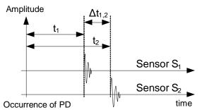
Figure 7: Absolute and relative times in a twosensor-setup
