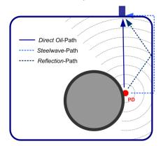
Figure 5: Possible propagation paths in the test object [18]
