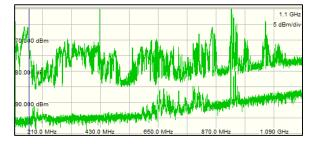
Figure 17: UHF Frequency sweep of the spectrum inside of the transformer and the measurement filter used shown as grey bar at 159.5 MHz
