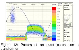
Figure 12 and Figure 13 compare the electrical PD pattern measured at the bushing tap of the one phase (Figure 12) and the synchronous reading of the UHF system, using a 1.5 MHz filter set to a center frequency of 490 MHz, inside the tank (Figure 13).
