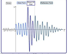
Figure 6: Acoustic PD signal components reflecting the propagation paths
