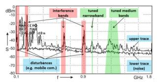
Figure 2: Signal relationships of proposed tuned UHF methods (schematic example) [10]
