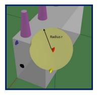
Figure 9: Spatial information from one sensor together with a UHF trigger
