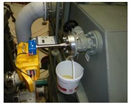
Figure 11: UHF sensor connected to the tested transformer in the factory test laboratory
