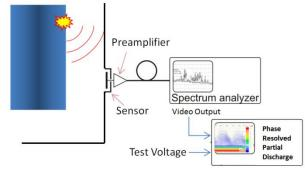
Figure 1: Example of a tuned UHF narrowband measurement with variable center frequency [9]
