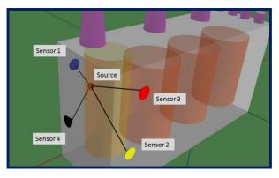
Figure 8: Principle of acoustic localization [18]
