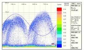
Figure 14: Pattern of internal PD inside a transformer [22]
