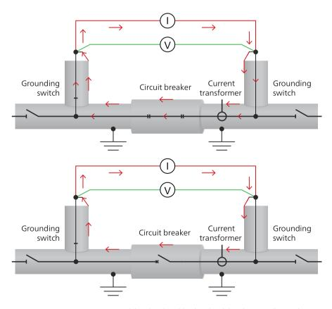
Contact resistance measurement with breaker closed (top) and with breaker open (bottom)
