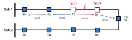
Figure 2: Fault location, isolation and service restoration in case of a fault
