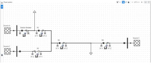
Figure 4: Example of Power System Model in RelaySimTest
