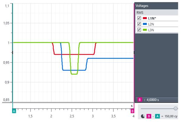
Figure 4: Test signal from reference measurement
