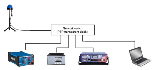
Figure 2: Test setup used for PQI testing: CMGPS (top), CMC 430 (left), SICAM Q200 (middle), CMC 256plus (right), Computer (own figure, source of individual pictures OMICRON [3] and Siemens [4]).
