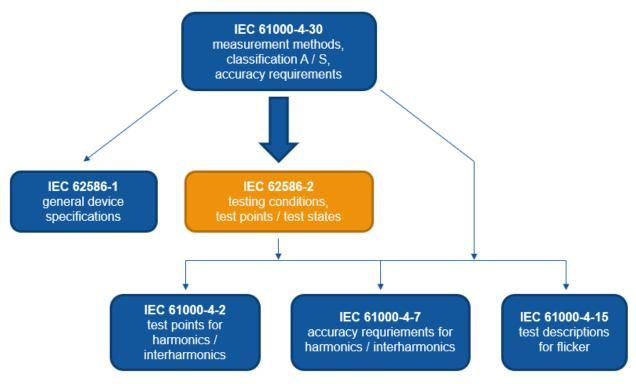
Figure 1: Framework of IEC standards for PQI testing
