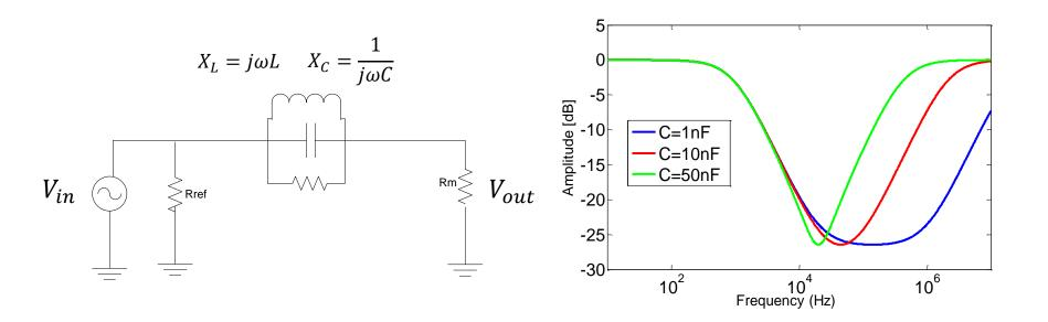
$\omega = \omega_{res}$ ,  $X_L = X_C$ , The Inductor and Capacitor Create an Open-Circuit at the Resonance Frequency!
