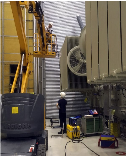
Figure 4. One time connection of the 3-phase transformer test system to perform all electrical tests according to Table 1.
