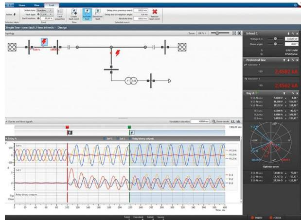
Figure 16: System-based testing with RelaySimTest
