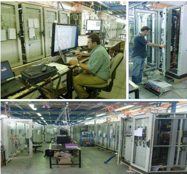
Figure 4: Factory test of a provisionally complete interconnected protection and digital control system
