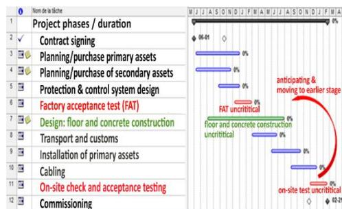
Figure 3: Simplified project plan and main project phases
