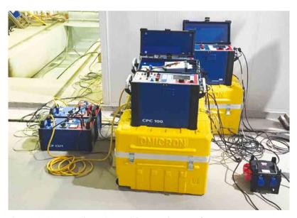
Three CPC 100 units with CPC Sync and three matching transformers were used for excitation of the dry type transformers.
