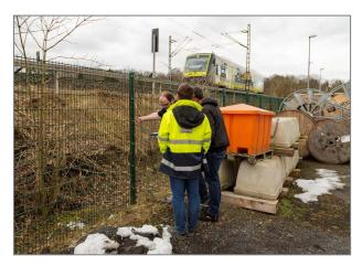
Figure 10 Step and touch voltage testing using COMPANO and HGT1
