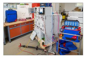
Figure 9 Primary injection into a current sensor
