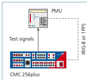
requirement is the synchronicity of the source and the PMU, which is established by time synchronization via GPS or IRIG-B. With GPS or IRIG-B add-on modules, synchronicity with a deviation of typically 1  $\mu$ s can be achieved when using a CMC test set for testing. In this case, the test signals are not only syn-
