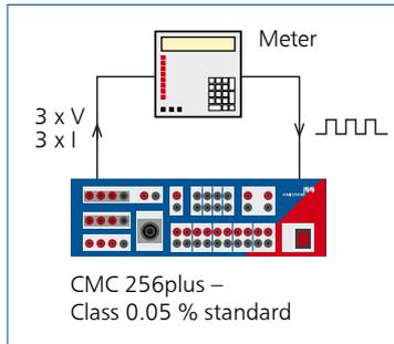
and current sources has been verified with measurements confirming the extremely low drift over a period of more than ten years. With cyclic calibration of the test set against a higher-level measurement reference, traceability to a national standard can be ensured.
