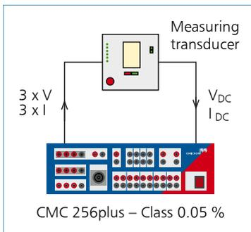
The operating software is tailored to these requirements and supports manual and automated testing of transducers with analog output signals of 0 - 10 V or 0 - 20 mA DC. The tests are performed using test tables with freely selectable test points. As a result, the software generates a test
