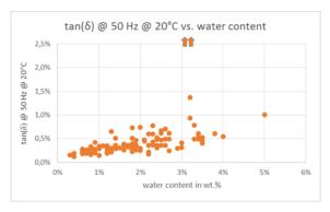
Figure 5. Ratio of  $tan(\delta)$  at 50 Hz and 20 °C to the water content in the cellulose at over 100 power transformers, assessed via broadband dielectric measurement using the OMICRON DIRANA test system. ( $tan(\delta)$  @ 50 Hz @ 20 °C vs. water content; water content in wt. %)
