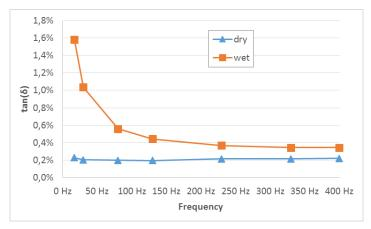
Figure 8. Frequency variable tan(ō) of a dry and a wet 33 kV OIP bushing at 30°C (data from [8]) (dry; wet)
