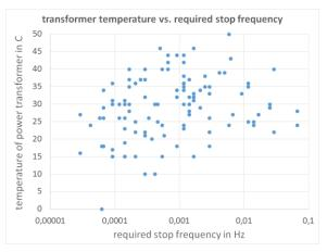
Figure 7. Required stop frequency, depending on the transformer temperature in a survey including over 100 power transformers (transformer temperature vs. required stop frequency; temperature of power transformer in C; required stop frequency in Hz)
