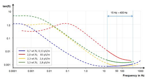
Figure 6. Broadband dielectric response of 4 different power transformers at 20°C. (Frequency in Hz)
