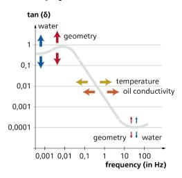
Figure 2. Dielectric properties of a power transformer oil-paper High- to the Low-voltage winding insulation (CHL)
