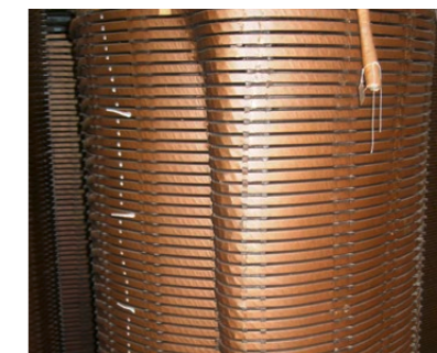
Buckling of winding
