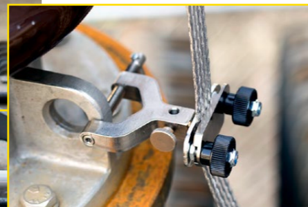
Flange-screw clamps with spikes function as reliable contacts even through layers of paint or dirt.
