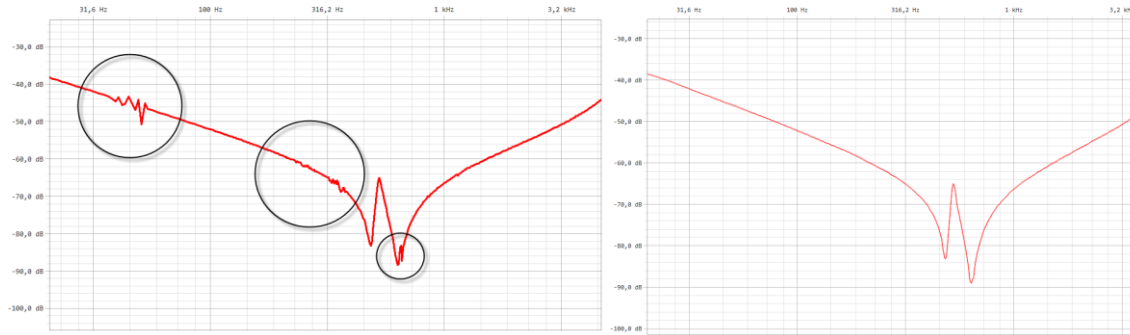
Figure 13: End-to-end open-circuit on HV winding performed with SFRA Instrument 1 (left) and SFRA Instrument 2 (right)
