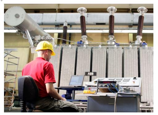
Partial discharge diagnosis of a power transformer
