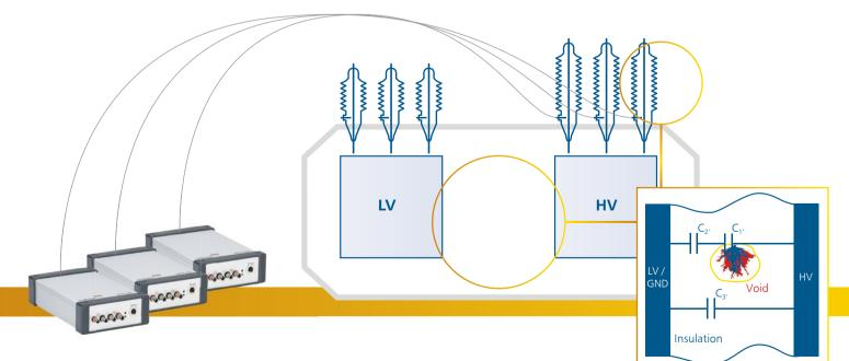
For synchronous multi-channel PD measurements, e.g. for three-phase testing, at least three MPD 600 acquisition units are needed for connection to the HV bushings.
