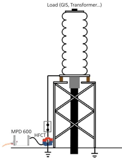
Basic connection diagram of HFCT at a cable end termination
