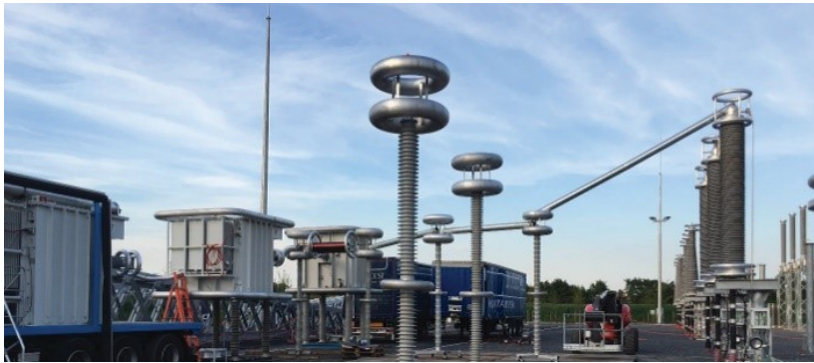
Figure 10. Resonance test set-up for testing of cable system
