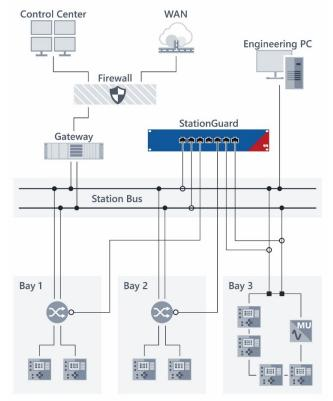
Figure 2 How IDS can be connected to the substation network
