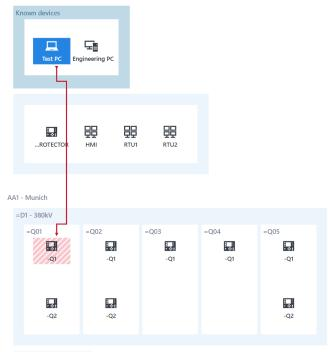
Figure 4 Graphical alarm display instead of event list
