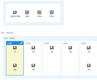
Figure 6 Maintenance mode activated for bay Q01
