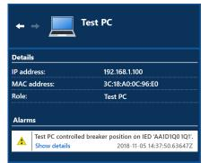
Figure 5 Details for Fig. 4: Test PC attempting unauthorized control of circuit breaker
