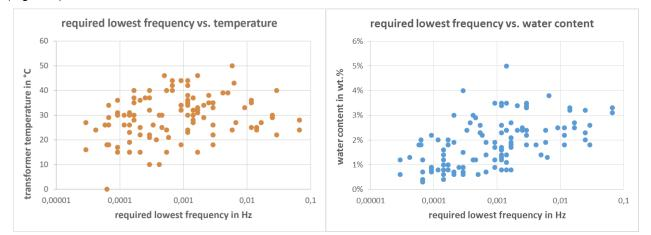
Figure 8: Correlation of transformer temperature and water content to the required lowest frequency which has to be measured. The evaluation is based on 115 dielectric measurements on power transformers.
