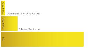
Test time for frequency sweep from 1 kHz to 10  $\mu\text{Hz}$
