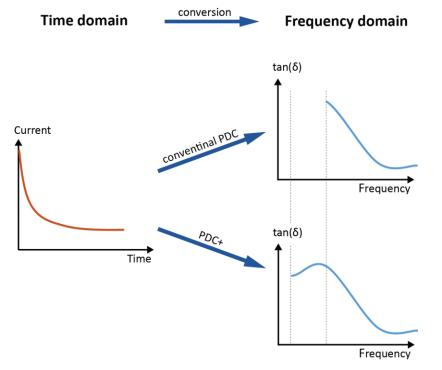
Figure 6: Conversion from time to frequency domain for conventional PDC and PDC+
