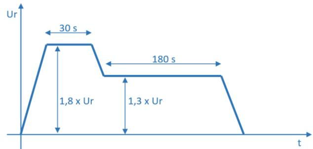
**Figure 2** PD measurement test cycle according to IEC 60073-11 [3].
