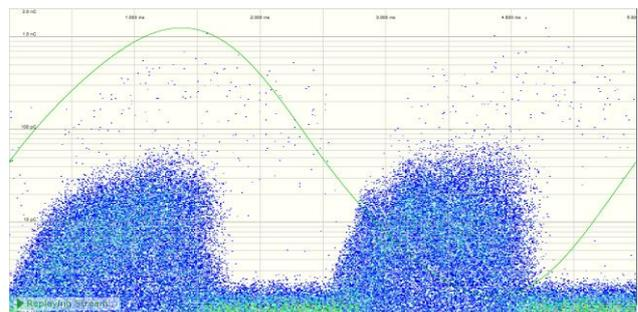
**Figure 8** Surface discharges on the HV winding.
