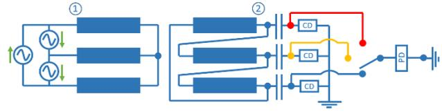
**Figure 1** PD measuring configuration according to IEC 60073-11[3].
