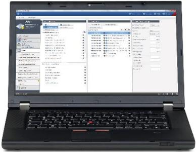
Based on the nameplate values, PTM generates a customized test plan according to current standards and guidelines for each asset.
