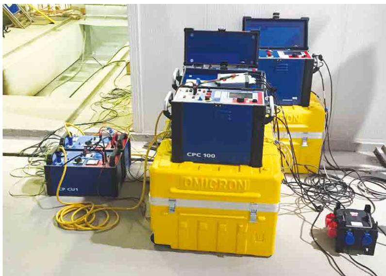
Three CPC 100 units with CPC Sync and three matching transformers were used for excitation of the dry type transformers.
