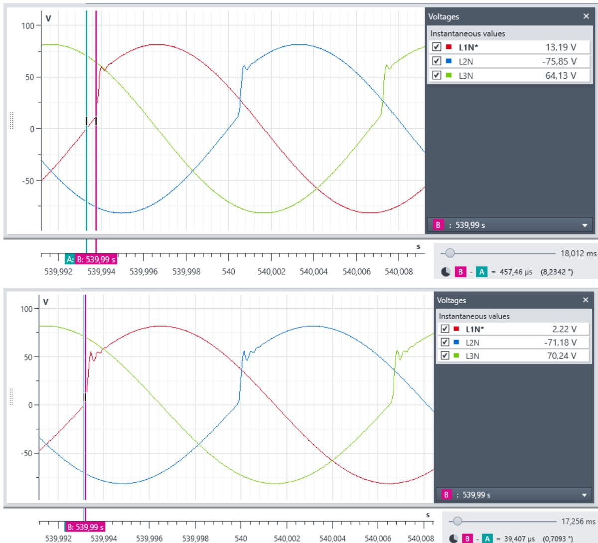
Figure 5: Output signals of phase jumps test; a) without appropriate rounding (upper); b) with appropriate rounding (lower)
