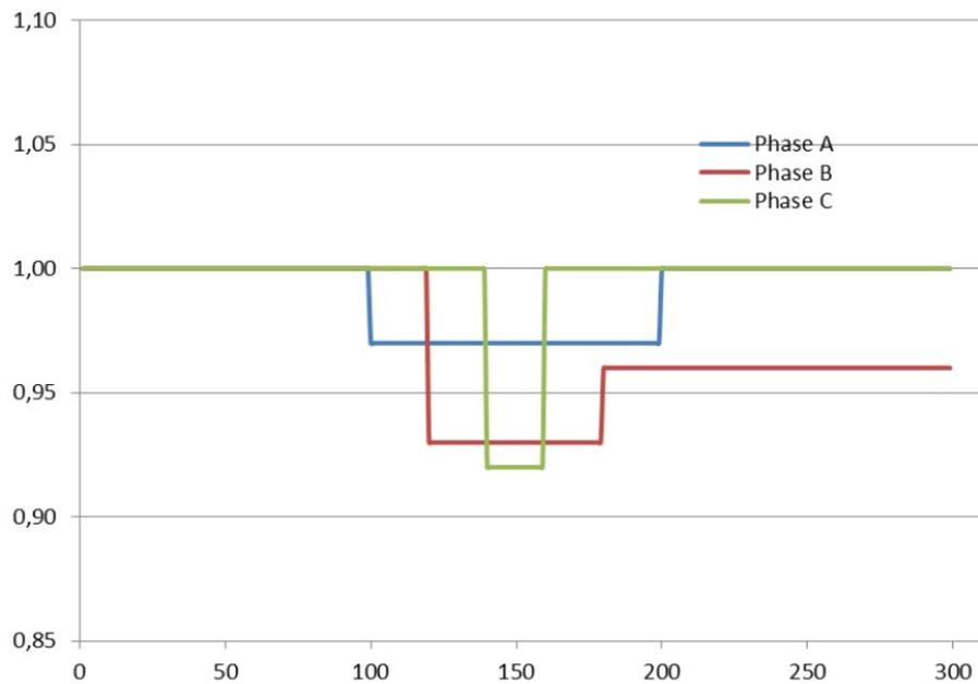
Figure 3: Test signal as described in the standard; x-axis time in half-cycles; y-axis: voltage in *pu* (source: IEC 62586-2 [5])
