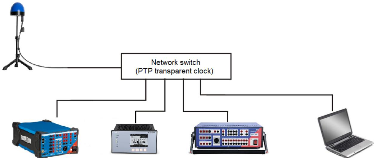
Figure 2: Test setup used for PQI testing: CMGPS (top), CMC 430 (left), SICAM Q200 (middle), CMC 256plus (right), Computer (own figure, source of individual pictures OMICRON [3] and Siemens [4]).
