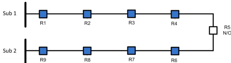
**Figure 1:** Typical feeder automation example with a tie recloser.
