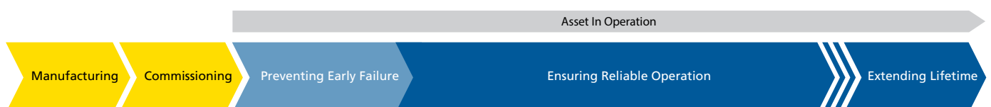
The integrity of the insulation should be confirmed with PD measurement and monitoring at all stages of an asset's lifetime.
