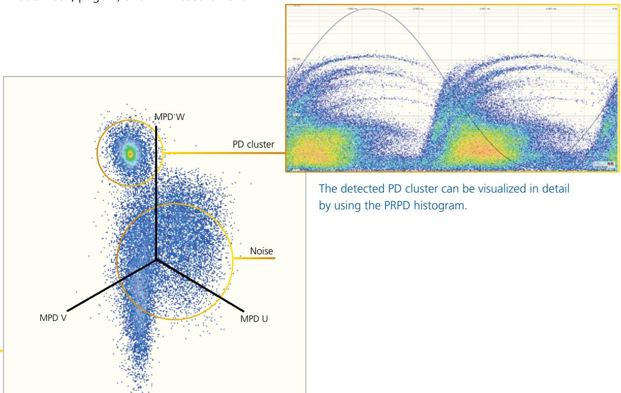
A 3PARD (3-Phase Amplitude Relation Diagram) separates PD sources from noise.
