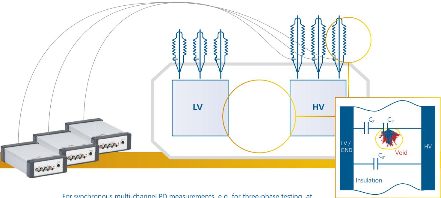
For synchronous multi-channel PD measurements, e.g. for three-phase testing, at least three MPD 600 acquisition units are needed for connection to the HV bushings.
