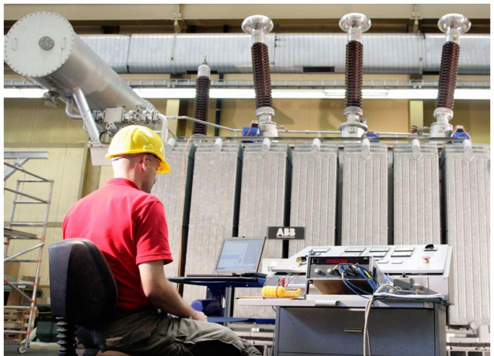
Partial discharge diagnosis of a power transformer
