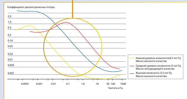
The dielectric response curve allows conclusions to be drawn about the different factors that influence the measurement result.
