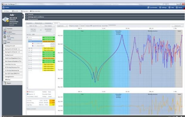
OMICRON's Primary Test Manager™ software offers automatic result assessment and comparison, also typical influences for deviations can be visualized.
