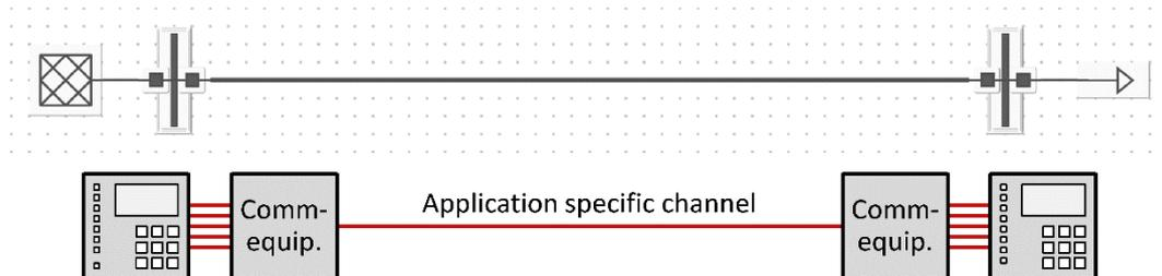
Figure 1: Conventional communication aided line protection scheme
