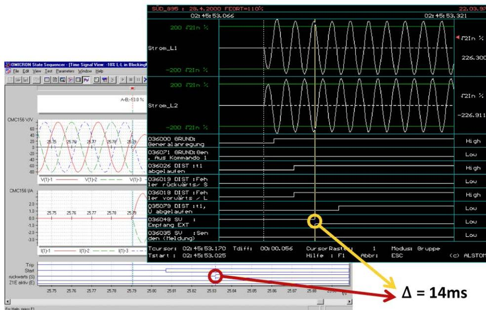
Figure 7: Transfer time of blocking signal evaluated from fault records
