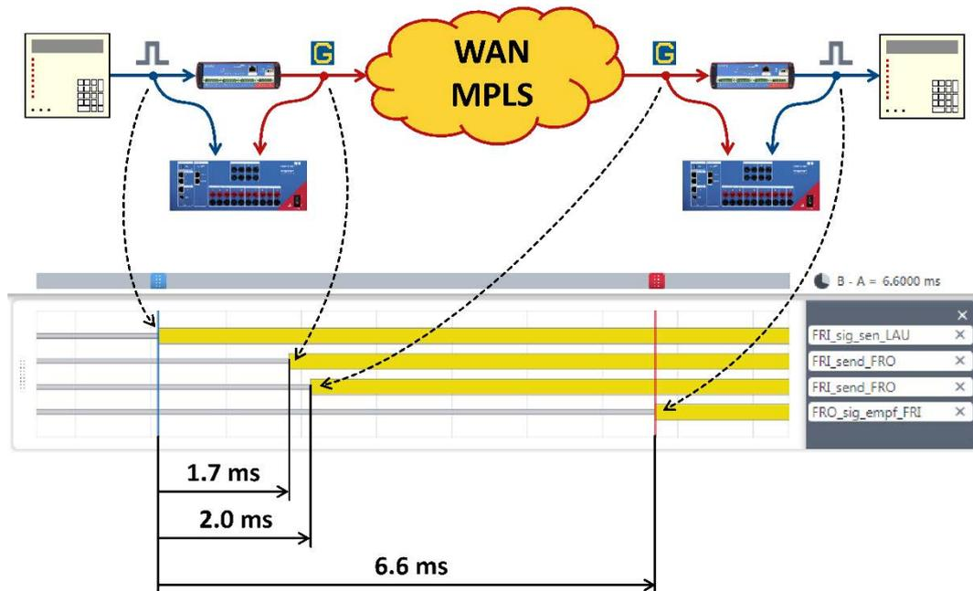
Figure 10: Signal propagation in the protection scheme
