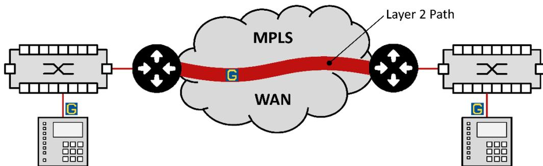
Figure 2: GOOSE communication between substations via a layer 2 path
