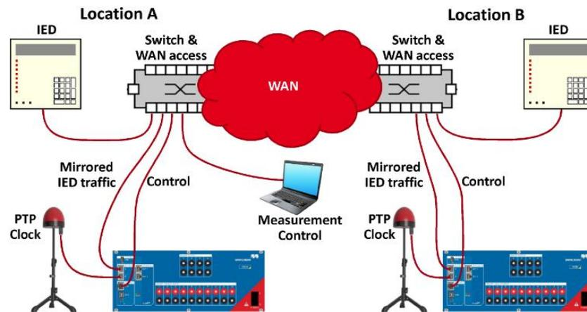
Figure 4: Propagation time measurement over a WAN
