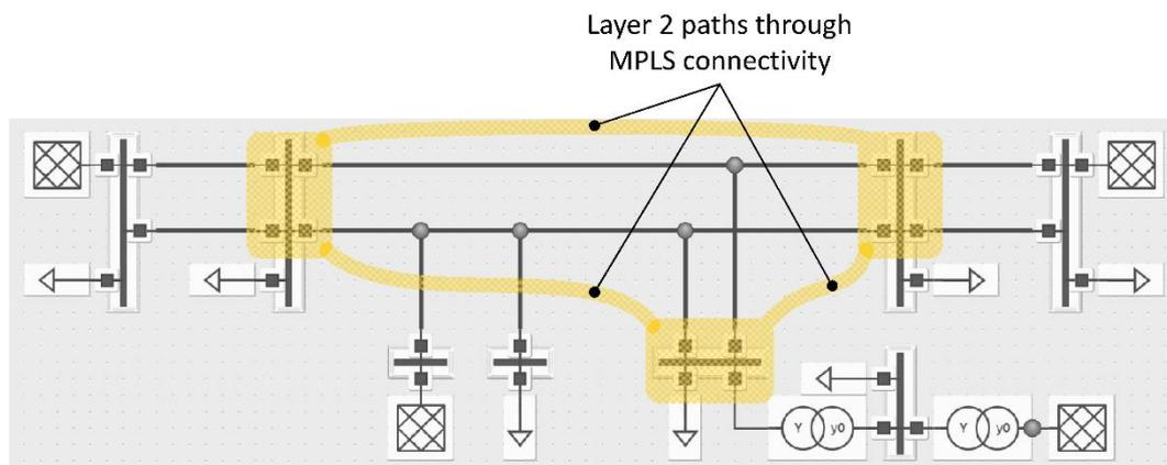
Figure 9: The IEDs in the three main locations in the scheme directly communicate via GOOSE
