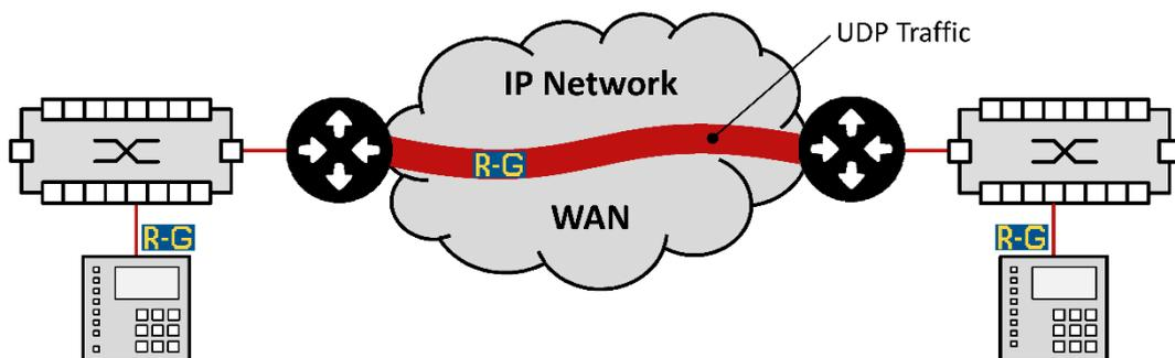
Figure 3: Routable GOOSE communication between substations via an IP route
