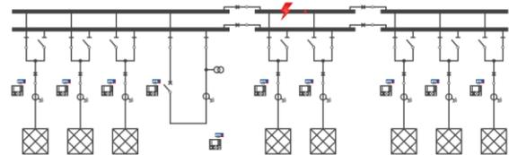
FIGURE 9: BUS FAULT ON MIDDLE SECTION
