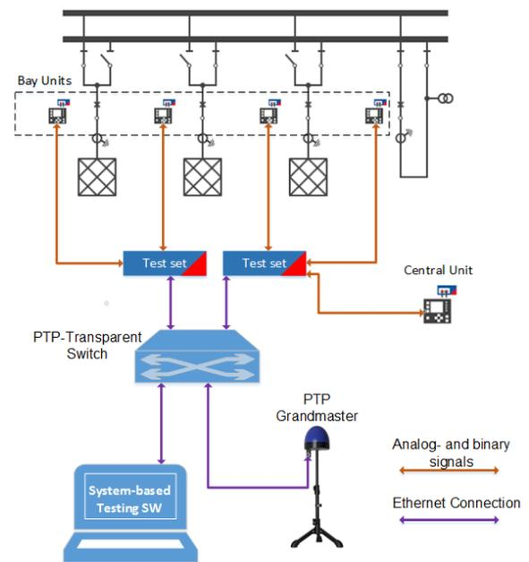
FIGURE 4 TEST SETUP FOR A SYSTEM-BASED BUSBAR PROTECTION TEST
