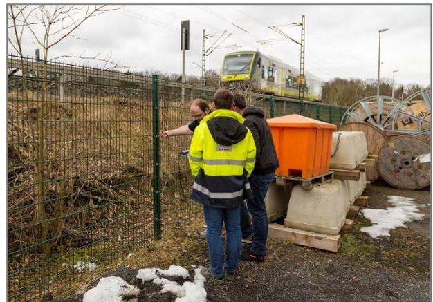
Figure 10 Step and touch voltage testing using COMPANO and HGT1
