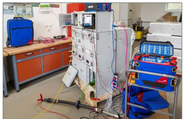
Figure 9 Primary injection into a current sensor
