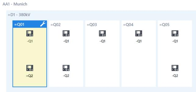
Figure 6 Maintenance mode activated for bay Q01
