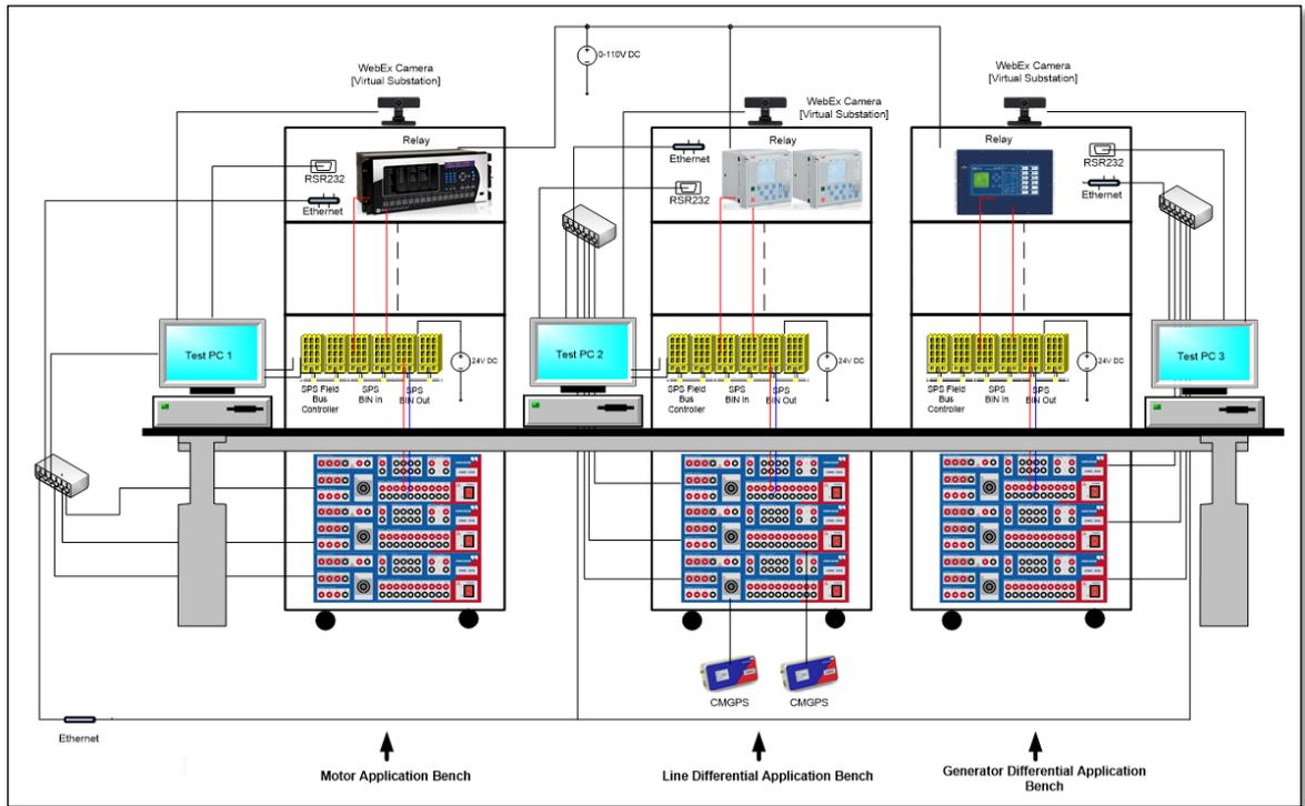
Figure 2: Concept for a relay test bench
