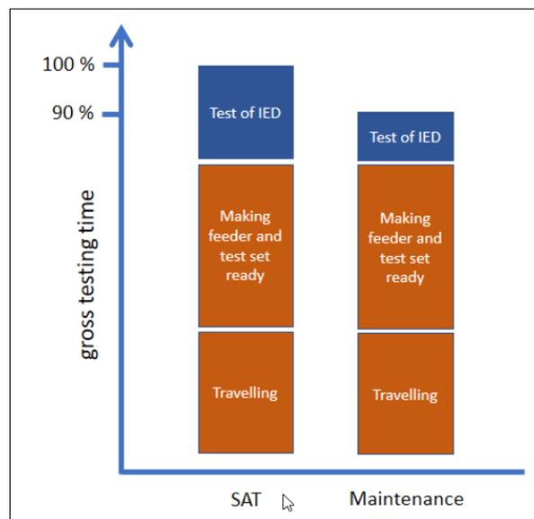
Figure 5: Comparison of gross testing time for SAT and maintenance testing
