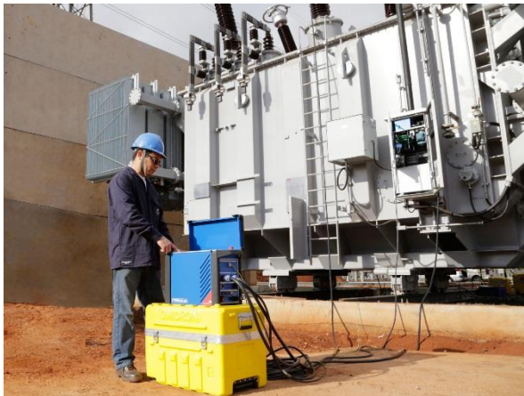
The integrated three sources and the simple wiring concept speed up and simplify power transformer testing.
