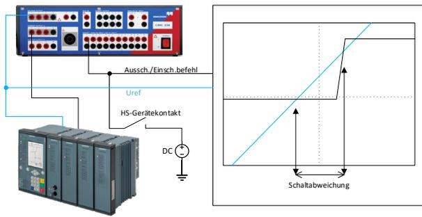
Figure 5 Measurement setup/principle
