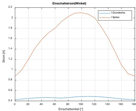
Figure 3: Maximum current as a function of the closing angle during 1-pole closing (L1:0°/L2:120°/L3:60°)
