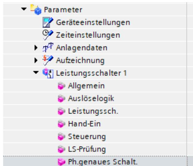
Figure 11b Point on wave switching parameter in Circuit Breaker function group
