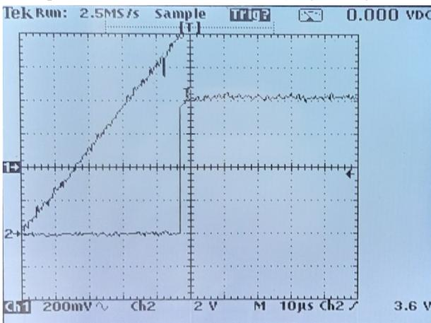
Figure 6 Measurement of closing time deviation
