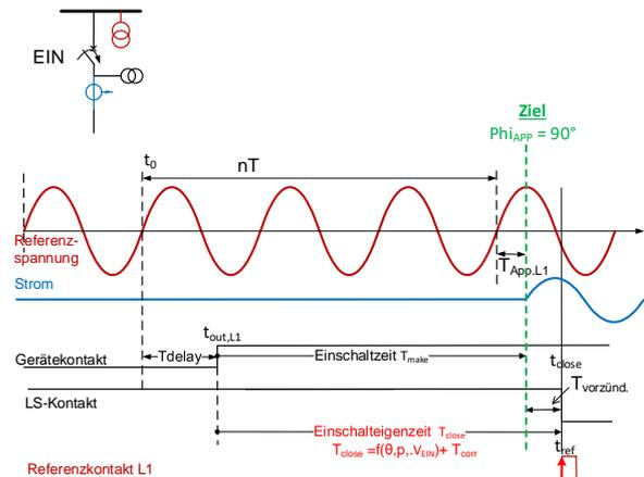
Figure 4: Principle of controlled switching
