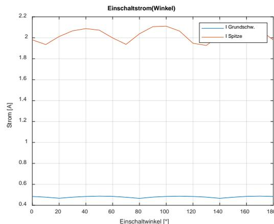
Figure 2: Maximum current as a function of the closing angle during 3-pole closing
