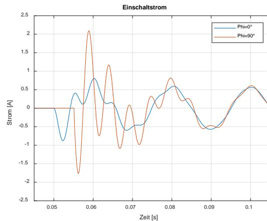
Figure 1: Inrush current at favorable and unfavorable closing angles in a MSCDN system
