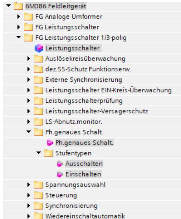
Figure 11a Point on wave switching in DIGSI 5 library
